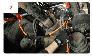
**Cradle the driveshaft.** Cradle the spring clip ratcheting rope assembly around the driveshaft. Ratchet the rope assembly tight to the drive shaft.
