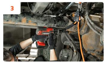
**Remove the driveshaft.** Remove the driveshaft, allowing the rope assembly to carry the weight.
