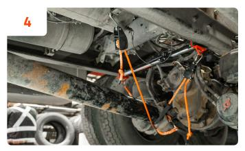
**Adjust for travel.** Using the ratchet, raise or lower the driveshaft into proper position. If offset placement is necessary, tie both spring clips into the same steel loop and adjust the height.
