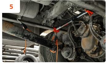
**Lateral securement.** Utilizing the hook-end ratcheting rope assembly, secure the ratchet hook end on a crossmember or frame rail of the truck. Wrap the spliced hook end of the rope between the u-joint and driveshaft – then hook back to itself. Ratchet the rope tight.
