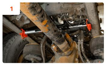
**Insert hanger bar.** Wedge the hanger bar between the truck's frame rails, making sure the padded C-brackets are tight against each lip. Close the handle so the spring loaded lock engages.
